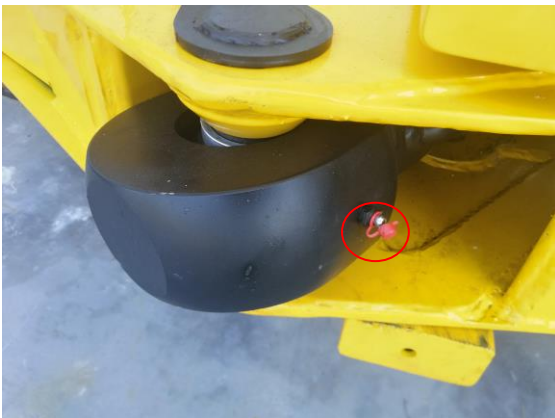
Figure 21 Grease the gripper bearings at the bottom and top
