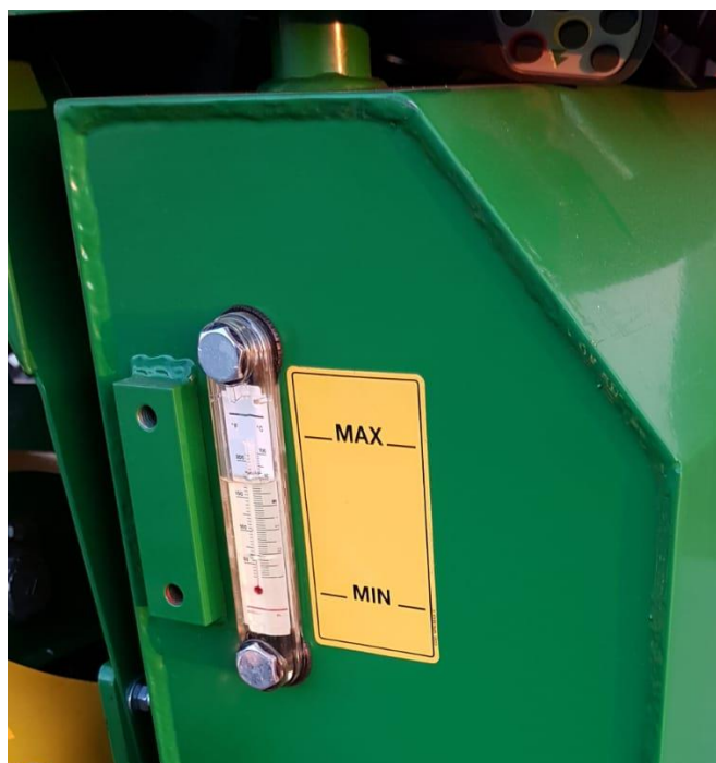
Figure 22MAX level and min hydraulic oil
