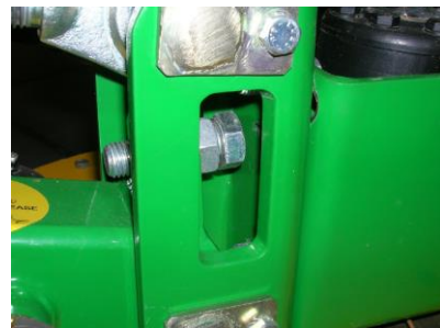
Figure 12 Brush minimum height adjustment
