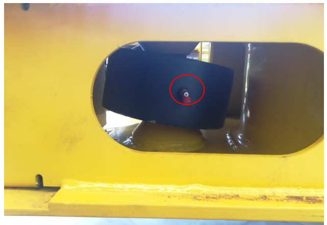
Figure 21 Grease the gripper bearings at the bottom and top
