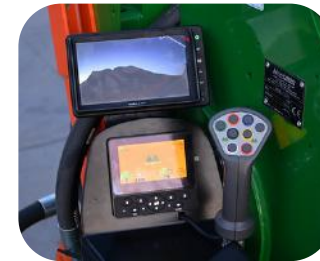
programmable joystick for self sequenced actions
