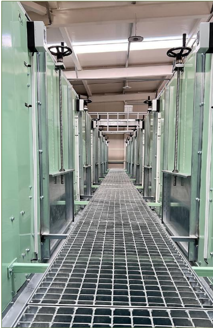
Two-leveled walking platform for easy access of the entire line
