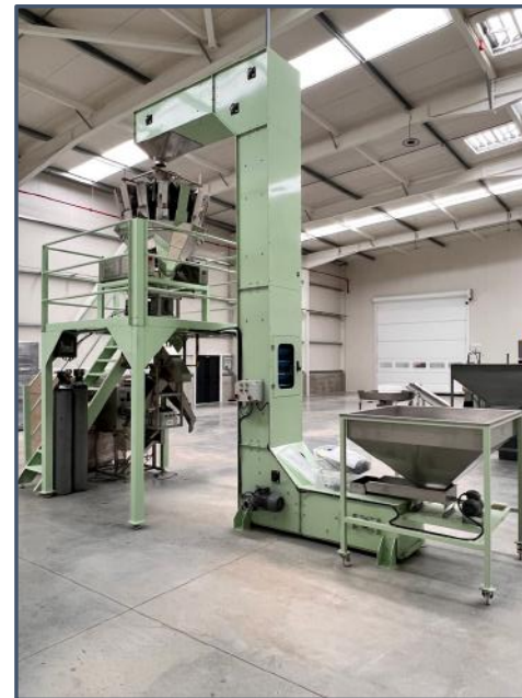
Stainless Steel bunker, food grade Z Elevator
