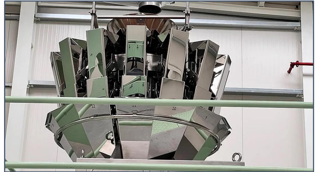
10 or 14 weighing heads, Stainless Steel
