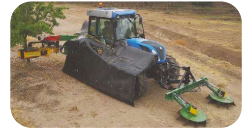
optional front brushes to avoid trampling of fruits
