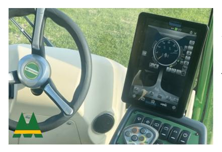
All cotrols at the tip of your finger using a multi-functional joystick and a touch screen monitor that helps you monitor all functions, including multiple cameras.
